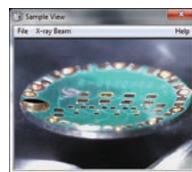
Camera view of a printed circuit board with the elliptical region of analysis shown at the center.
